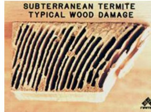
Fig 7. Subterranean termite damage.
